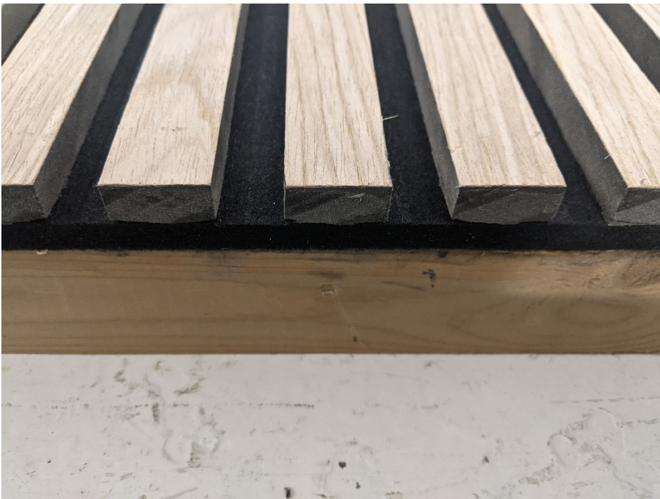
Figure 2 – Detail of specimen materials, as installed over furring strips
